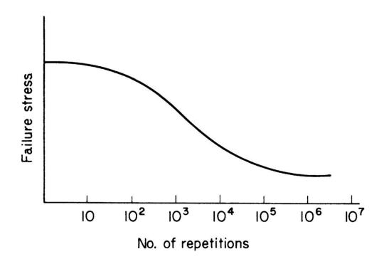
**FIGURE 13.2** Typical Form of *S–N* Diagram
